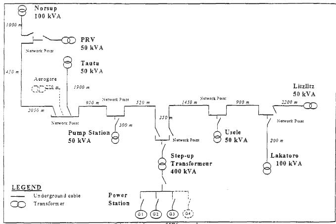
Schematic layout of HV network
