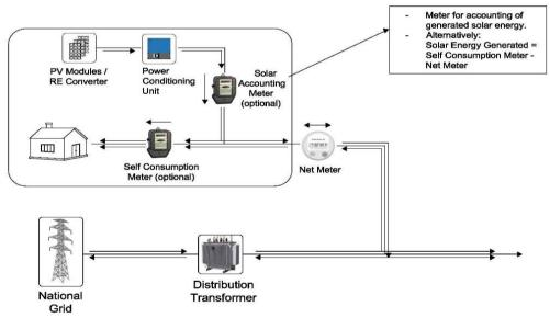
Figure 1: Typical net metering architecture.
