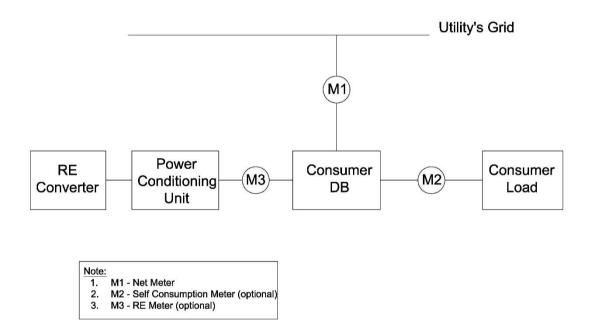
Figure 3: Schematic diagram of indirect connection to the grid
