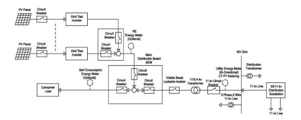
Figure 5: Type B connection [MV Consumer]
