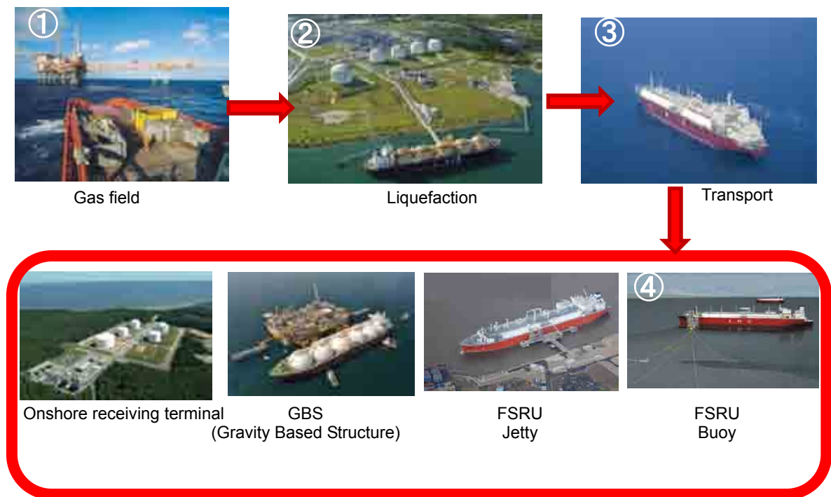
Fig. 5-8 LNG chain and receiving terminal
