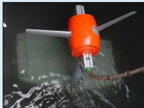
Figure 16 - 10 kW micro hydro turbine at Bhira
